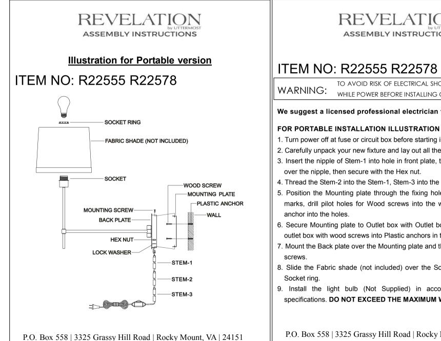
ITEM NO: R22555 R22578 TO AVOID RISK OF ELECTRICAL SHOCK, BE SURE TO SHUT OFF WHILE POWER BEFORE INSTALLING OR SERVICING THIS FIXTURE. We suggest a licensed professional electrician for installation
